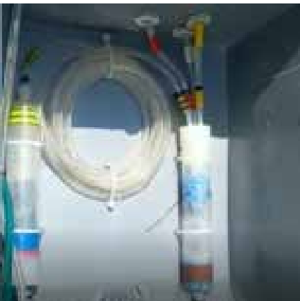
Figure 35 - The FaRAGE in action: Water and atmospheric air are mixed in the left syringe and the tube. From the right syringe, gas is pumped to the gas analyzer and the water discharged.
