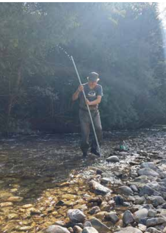
Figure 38 - Steven Weiss taking field measurements of river width, depths, substrate size and water flow with a point-transect approach.
