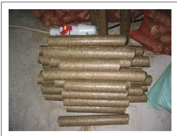
Figure 11. Briquettes made by using the reed in the Narew area (Source: Jutta Krumnacker)
